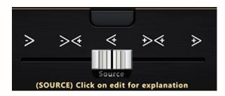
To understand source control, let's first explain what a source in the program is. The source is the place where the sound radiates from. All sound produced in the reverberation radiates from this starting point. With source control, we can control not only which way the source is facing but also its phase.
