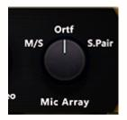
1. M/S: Mid side captures allow the user to create a stereo effect without issues when the image is collapsed to mono. In this version of M/S I used an omni as the centre and a figure 8 for the sides.
